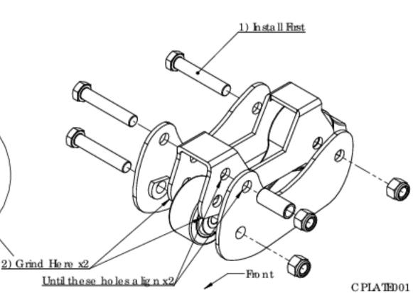
4) Only tighten assembly after vehicle has been lowered to the ground.
