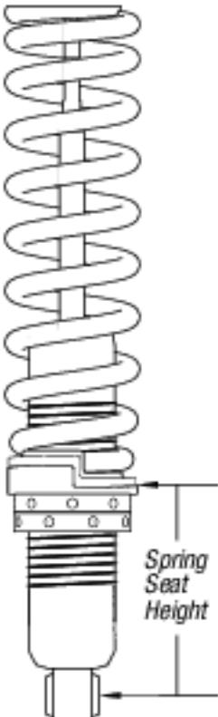
Foam Cell Pro Struts feature a threaded body for ride height adjustment.
